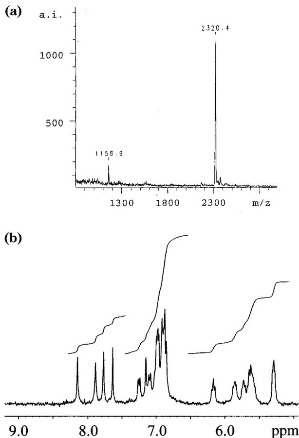
**Figure 4.** Selected spectra of purified **24**: (a) MALDI-TOF spectrum showing both  $[M - H]^-$  and  $[M - 2H]^{2-}$  ions, (b) nucleobase and H1' region of the  $^1\text{H}$  NMR spectrum in  $\text{D}_2\text{O}$  at 300 MHz and 22 °C.
