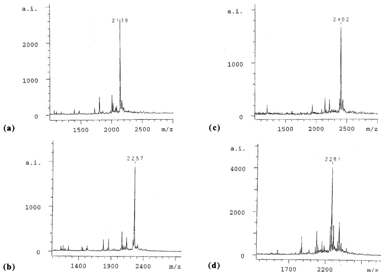
**Figure 3.** MALDI-TOF mass spectra of crude products obtained with optimized procedures: (a) **29**; (b) **31**; (c) **30**; (d) **32**.
