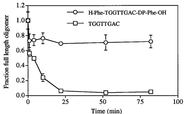
**Figure 6.** Nuclease stability of 3',5'-dipeptidyl-hybrid. Kinetics of nuclease degradation of **35** and its unmodified DNA counterpart 5'-TGGTTGAC-3' by snake venom phosphodiesterase (EC 3.1.4.1), as measured by MALDI-TOF mass spectrometry.
